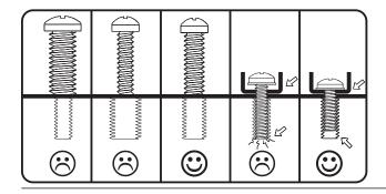
The back of your TV has 4 screw holes in a square or rectangular pattern. This is where the mount will attach to your TV. We provides several sizes and lengths of screws. This guide will help you select the right screws for your TV. You will only use 4 of the provided screws to attach your TV – the rest are not needed.
