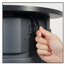
3. Secure 4 underside latches to hooks attached to shipping case.
