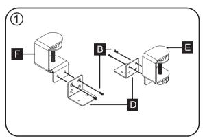
Attach C-clamp to the L shaped parts using the screws B provided at desired height
