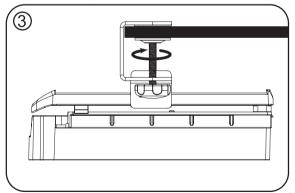
Turn the knobs on the C-clamps to secure the keyboard tray to your desk.
