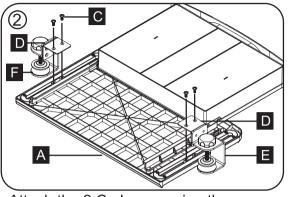
Attach the 2 C-clamps using the screws C provided.
