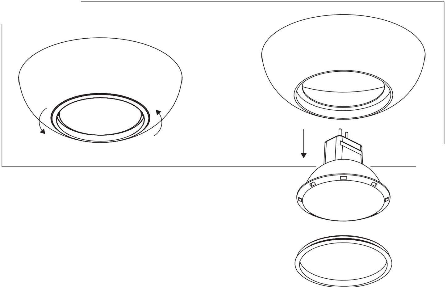
Place new LED in position and reverse the steps to connect the new LED.
