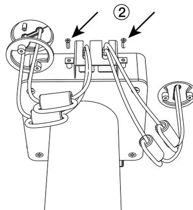
② Unscrew the 2 screws on cable cover.
