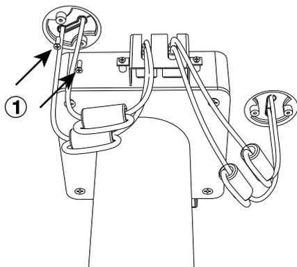
① Detached the cable clip by unscrewing the 2 screws.
