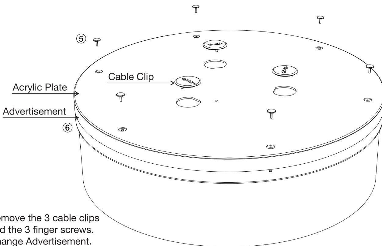
⑤ Remove the 3 cable clips and the 3 finger screws.
