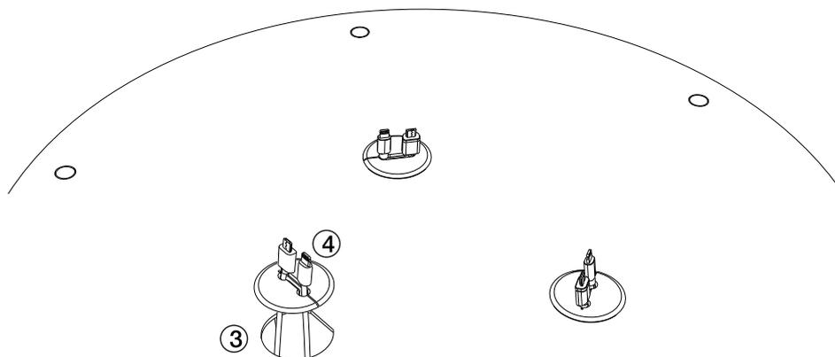
③ Remove cables from cable clip.
