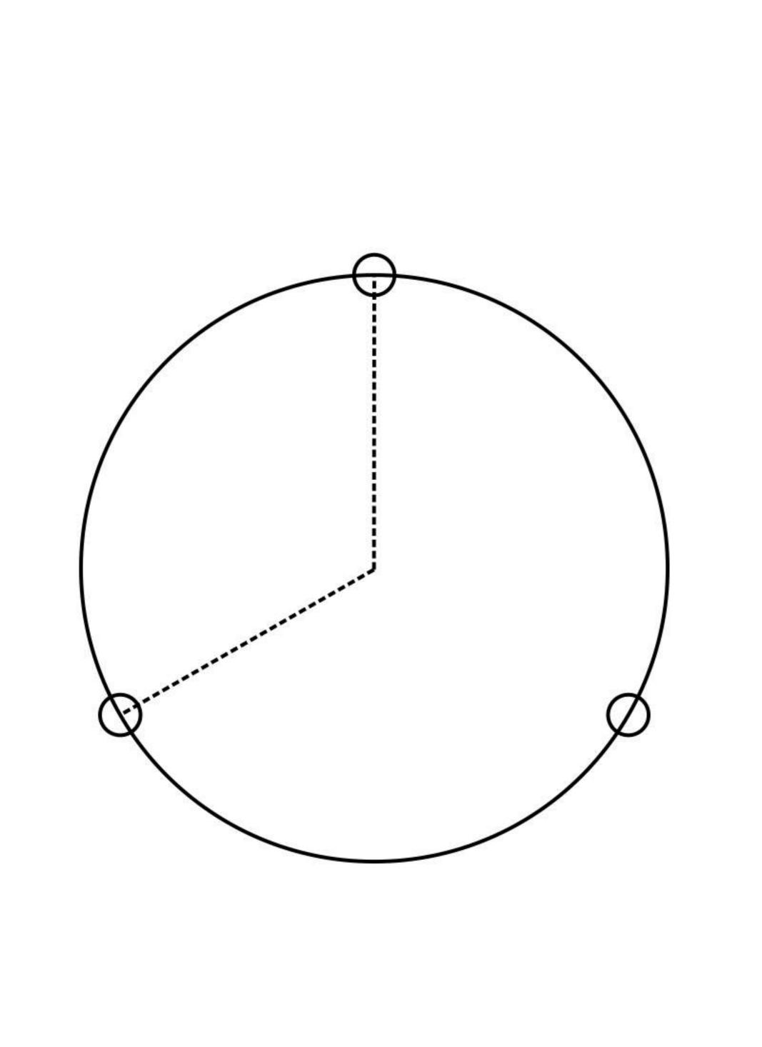
Mark the position of the holes on the ground. Drill the holes in using an impact drill.
