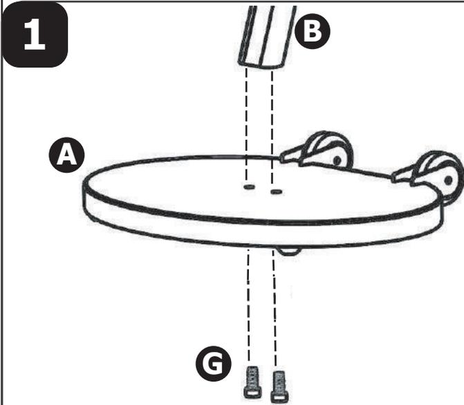
Attach post to base using M8 socket head screws. Use supplied hex key.
