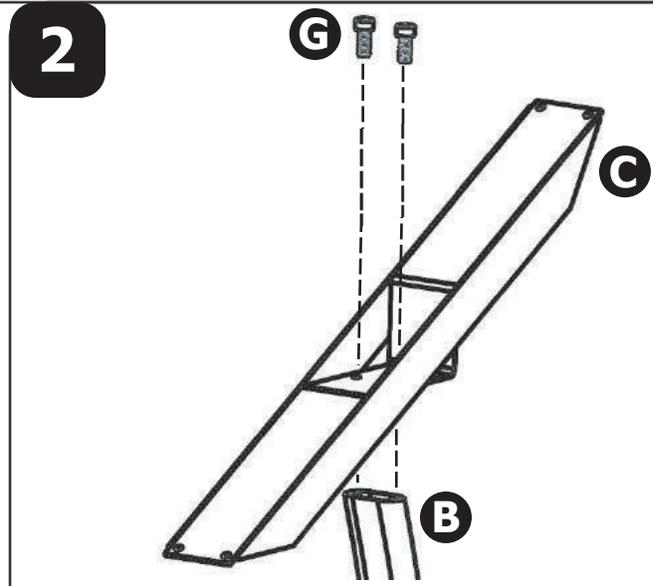
Attach mounting bracket to post using M8 socket head screws. Use supplied hex key.
