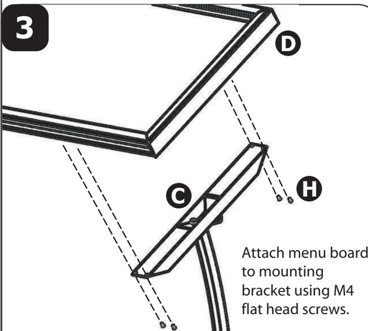
Attach menu board to mounting bracket using M4 flat head screws.
