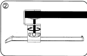
Turn the knobs on the C-clamps to secure the keyboard tray to your desk.
