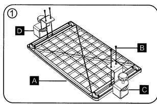
Attach the 2 C-clamps using the screws provided.
