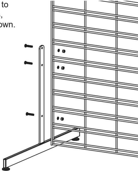
2. Connect the second Leg to the other side of the Gridwall as shown.
