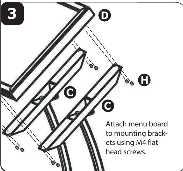
Attach menu board to mounting brackets using M4 flat head screws.
