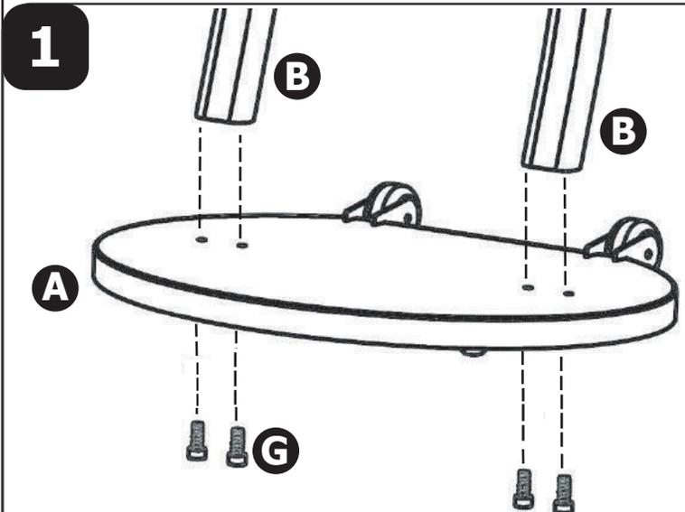
Attach posts to base using M8 socket head screws. Use supplied hex key.
