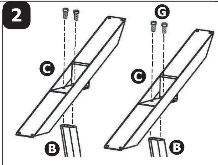
Attach mounting brackets to posts using M8 socket head screws. Use supplied hex key.
