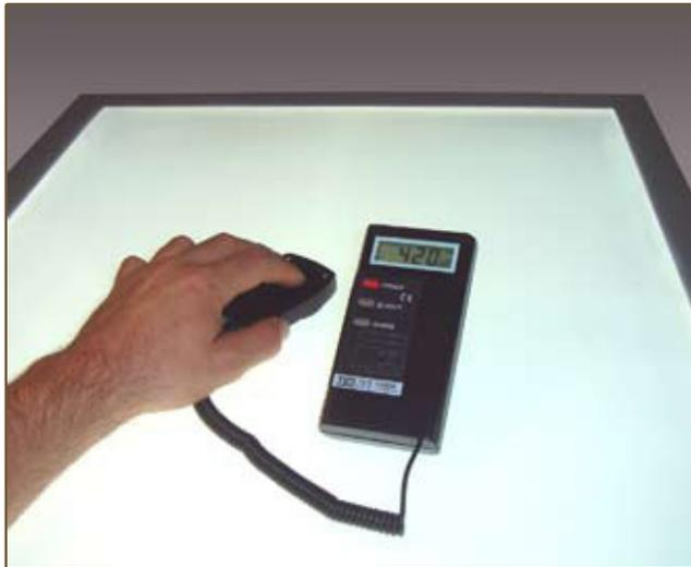
Nine readings are taken across the surface of a panel, the average of these readings being the average luminance of the panel. It is important to note that the figures for the centre of the light panel are slightly higher, meaning that graphics are slightly brighter in the centre.
