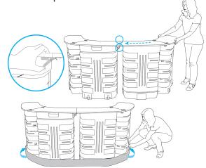
3. Move 2 assembled cases next to each other and join them by locking the latches underneath the countertops. Wrap PVC kickplate around the bottom to cover wheels. Attach the hook and loop strips on the ends of the kickplate to the corresponding pieces inside the case.
