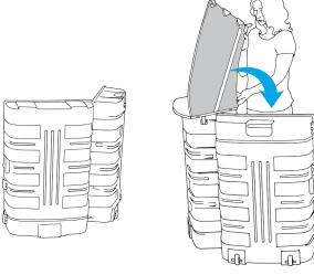
1. Stand shipping case upright, unlock the 4 clips and open the case. Lift up countertop latches. Align underside groove with shipping case edge and rest in place.
