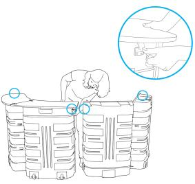
2. Secure 4 underside latches to hooks attached to the side of the case. Repeat step 1 & 2 on the other side.
