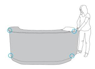
4. Wrap the fabric from the bottom and stretch to cover the counter top. Insert shelves at the designated slots inside the case.
