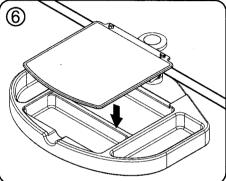
Insert mouse tray onto the center slot as shown in the picture
