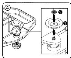
1 Place the metal plate on the screw
