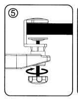
Tighten the screw to secure the tray onto a desk
