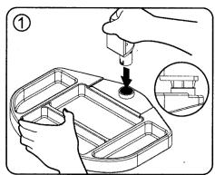
Forcefully insert C-clamp into the hole on the tray as shown in the picture
