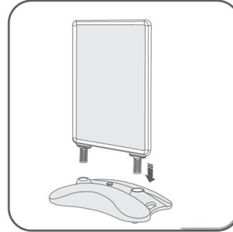
**2** Insert the spring legs into the holes in the heavy duty base
