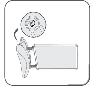
**3** Tilt the unit over. Tighten the bolt supplied to fix the frame to the base
