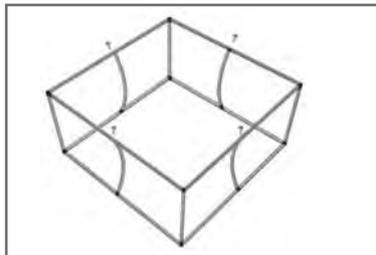
Attach 4 sets of Long Bars on the assembled frame, using the remaining Short Screws (D) to fix the Curved Side Support (E). Align the corners but do not attach.
