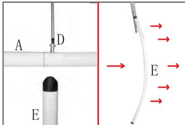
Align each Curved Side Support (E) with the holes in the center of each side, make sure the curve of the Curved Side Support (E) towards the center of square. Then, attach Short Screws (D) as image.
