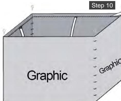
Zip the Graphic closed all the way around. Finally, connect the wire rope (F) to the loops of Eyebolt (C).
