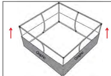
Unzip the Graphic all the way around, then push the blank back side of graphic under the bottom frame. With the help of another person, position your graphic, ensure the graphic is facing front-side out. Then, raise the graphic up.
