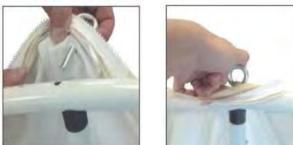
Find the reinforced hole in the Graphic that is nearest to the zipper ends. Feed a Eyebolt (C) into the top hole of Short Bar (B), then hand tighten.
