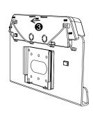
Open the front panel by unscrewing the five (5) screws.
