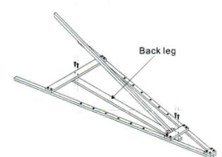
STEP2. Connect the back leg through the connecting plate A and B with screws, tighten them with Allen key, as shown above.
