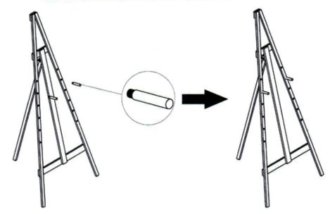
STEP3. Screw pegs into the front feet at the desired height. Assembly is finished.
