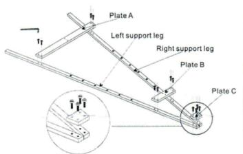
STEP1. Assemble the left support leg and right support leg through the connecting plate A,B,C with screws and tighten them with Allen key,as shown above.
