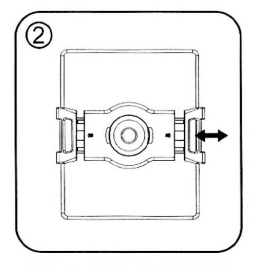
Pull open the bracket over the tablet and release
