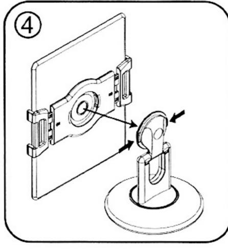
Press buttons, attach bracket, release buttons, and spin until you hear the click
