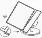
Insert sleeve peg into bottom hole of support bracket.
