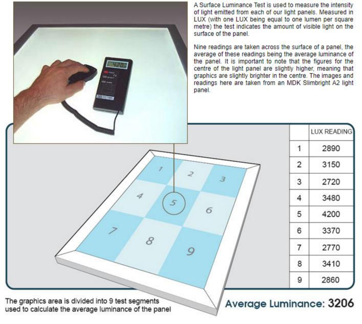
Using the light metre to measure the the centre position (see reading for position 5) of an MDK-A2. The light metre measures in foot candles (fc) - one foot candle being equal to 10 LUX, thus the reading of 420 fc equates to 4200 LUX.
